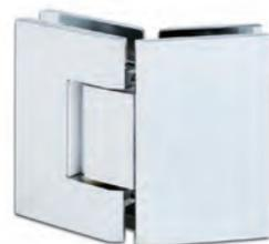
**i** Mounting: Glass/Glass 135° · Door opens both ways 90° · Distance Glass/Glass 5 mm · Glass thickness 8, 10, 12 mm
