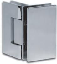
❗ Mounting: Glass/Glass 90° · Door opens both ways 90° · Distance Glass/Glass 11 mm · Glass thickness 8, 10, 12 mm
